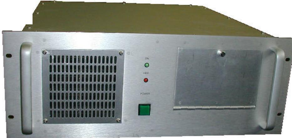
This is the most commonly used model for rack mount PC. All cables and wires are connected in the back of the chassis. A 3.5 disk drive mounting kits and HDD door covers are included. Motherboard sits on a universal mounting plate for easy removal. A 12VDC fan is mounted behind front panel with filter to intake air and to pressurize inside to prevent dust entering.
